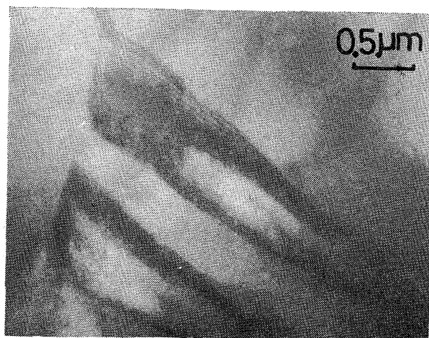
Photo. 2. Clustering of tangled dislocations of 304 steel hydrogenated at 400°C under 270 atm for 250 h.
