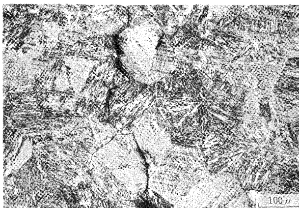
Photo. 4. Grain boundary crack propagation of temper embrittled alloy after tensile test at -125^{\circ}\text{C} (steel I).
