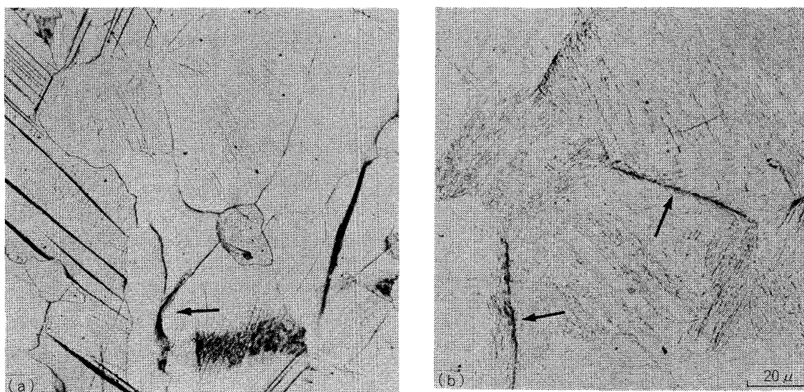
Photo. 3. Surface micro-crack initiation of temper embrittled alloys after tensile test at -196^{\circ}\text{C} .
