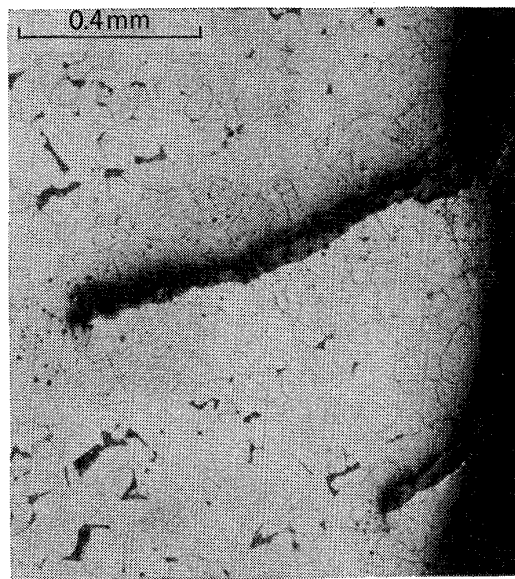
Photo. 2. Microstructure of seam-defects of the beam-blank.
