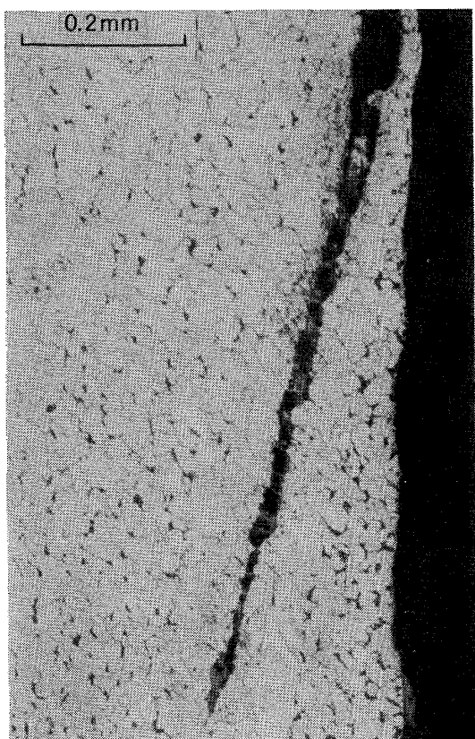
Photo. 1. Microstructure of seam-defects of the product.
