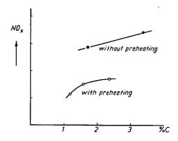
Fig. 1 Influence of the carboncontent with and without preheating (750°C) on the balance of returns with various amounts of return fines.
