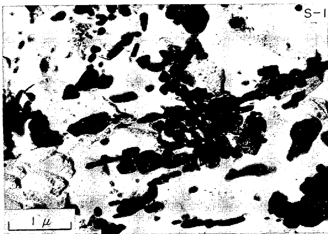
Photo. 6. Electron micrographs of specimens quenched at 1150°C for 1/2 hr and tempered at 700°C for 1000 hr (extraction replica).
