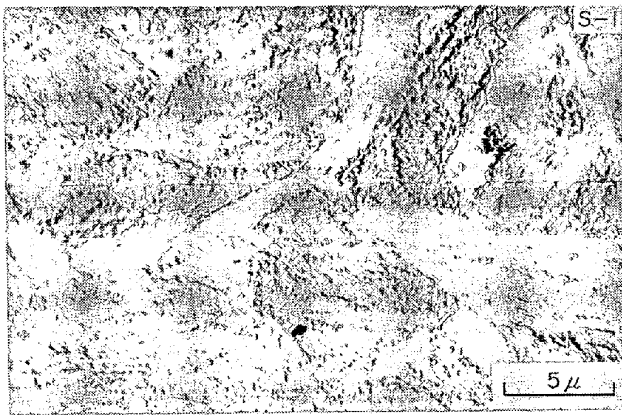
Photo. 1. Electron micrographs of specimens quenched at 1 150°C for 1/2 hr and tempered at 700°C for 1 hr (replica).
