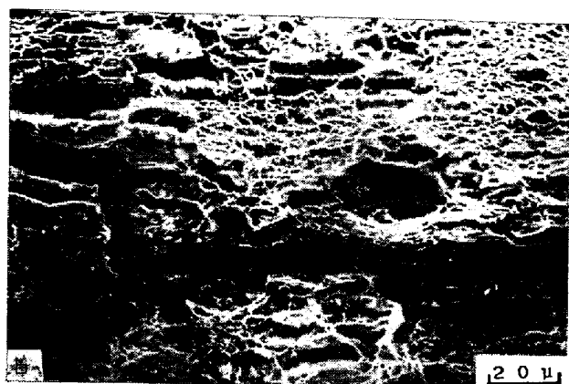
(a) Dimple pattern. Fractured by 47% tensile strain at 0^{\circ}\text{C} . \theta = 45^{\circ} . (b) Cleavage cracks. Fractured by 47% tensile strain at -196^{\circ}\text{C} . \theta = 0^{\circ} .
