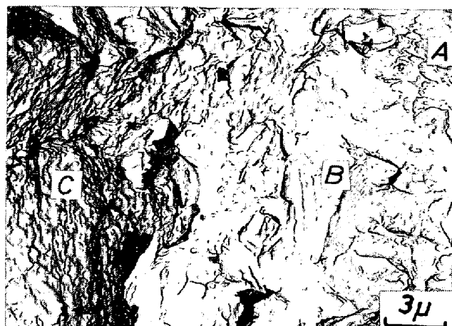
Photo. 1. Typical electron microfractograph of macroscopic brittle fracture surface of temper embrittled steel after Charpy impact test, A : Ductile, B : Quasi-cleavage and C : Intergranular.
