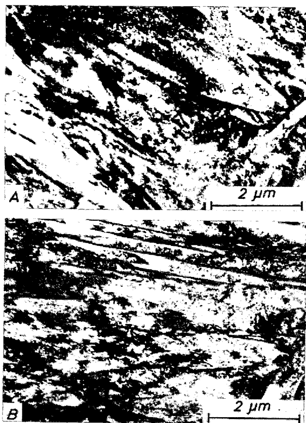
A) Steel No 2, austenitized at 850°C and oil-quenched. B) Steel No 2, austenitized at 1250°C and oil-quenched after holding at 850°C.
