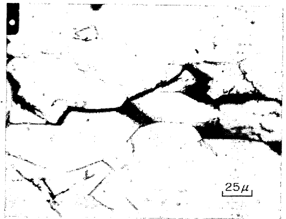
Photo. 5. Intergranular fracture on A-2-H in 42% MgCl 2 solution with 45.3 kg/mm 2 stress. Time to fracture : 1.69hrs.
