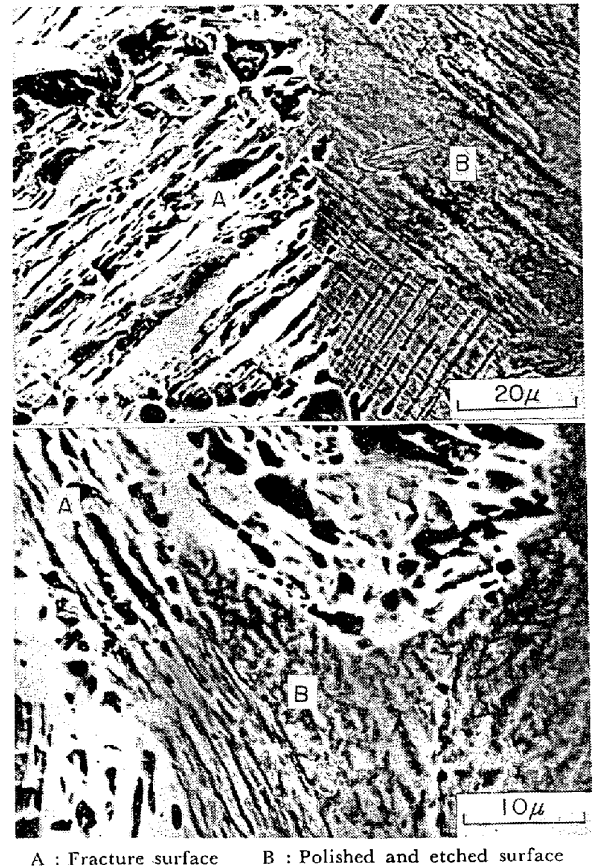
Photo. 4. Scanning electron micrographs of 2mm V notch charpy impact specimens in 350 grade 18%Ni maraging steel ( 1150^{\circ}\text{C} \times 1\text{hr WQ} + 510^{\circ}\text{C} \times 3\text{hr AC aged} ).
