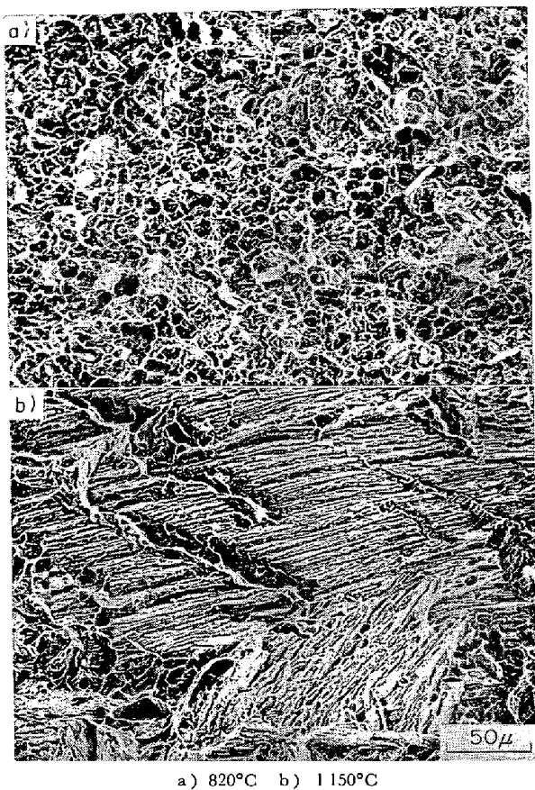
Photo. 3. Scanning electron micrographs of 2mm V notch charpy impact specimens in 350 grade 18%Ni maraging steel ( T^{\circ}\text{C} \times 1\text{hr WQ} + 510^{\circ}\text{C} \times 3\text{hr AC aged} ).
