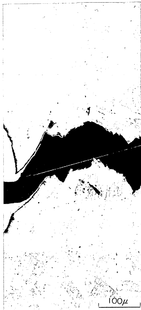
Photo. 13. Optical micrograph of fracture profile of 2mmV notch charpy impact specimen in 300 grade 18%Ni maraging steel ( 1150^{\circ}\text{C} \times 1\text{hr WQ} + 490^{\circ}\text{C} \times 3\text{hr AC aged} ).
