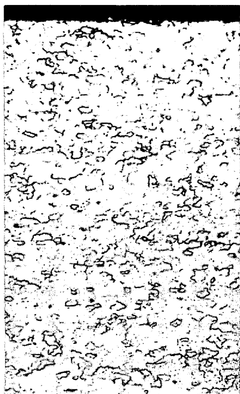
(a) Batch-annealed at 780°C for 1 hr (G.S. No. 8·7)
