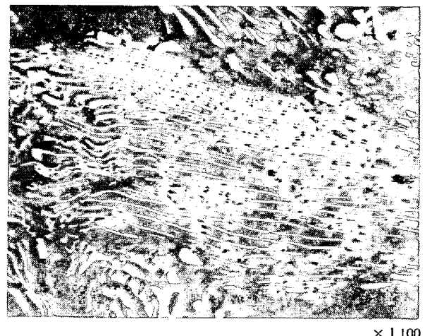
Photo. 8. Early stage of void initiation within pearlite nodule in the specimen spheroidized at 790°C, strained to \epsilon=0.84 .
