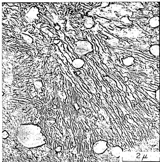
Photo. 2. Microstructure of inverse quench-hardened area in Fig. 1.
