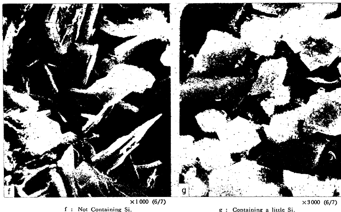
Photo. 6. Scanning electron microphotograph of aluminate inclusion extracted from Al killed steel (steel No. D).
