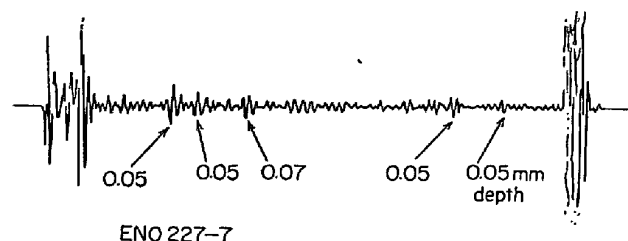
Fig. 4. Record of flaw signals for austenitic stainless steel wire rod without vibration.
