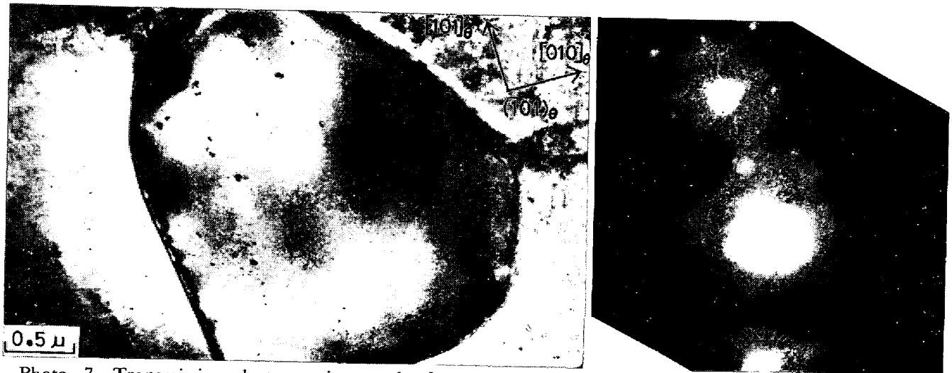
Photo. 7. Transmission electron micrograph of cementite in 1.25%C steel annealed for 5hr at 700°C after 92% cold-rolling showing the perfect annihilation of defect structures.
