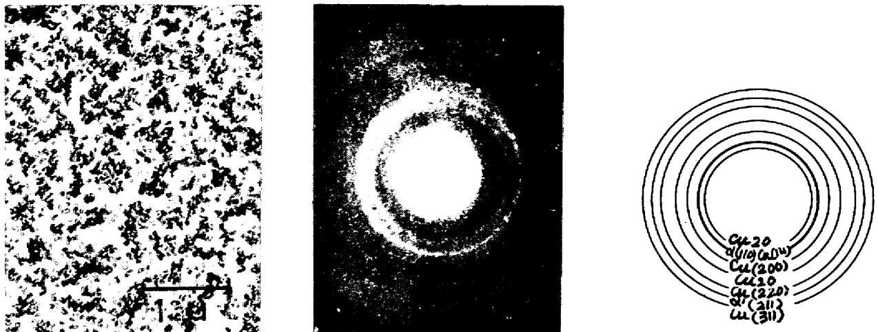
Photo. 6. Extraction replica image and electron diffraction pattern of steel No 1 aged at 525°C for 100hr.
