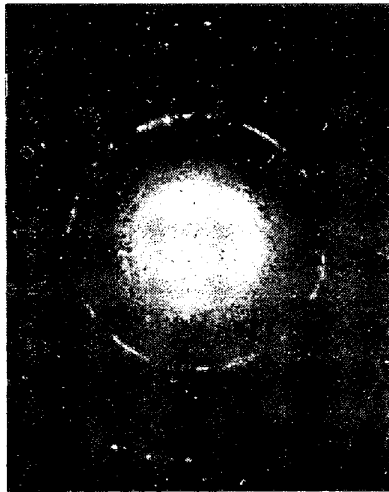
Photo. 4. Extraction replica image and electron diffraction pattern of steel No 1 aged at 525°C for 100hr.
