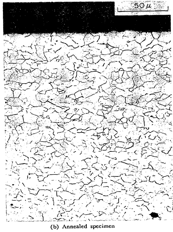
Fig. 8. Grain structures of hot bands coiled at 710°C and specimens annealed under heating cycle Y in Fig. 2.
