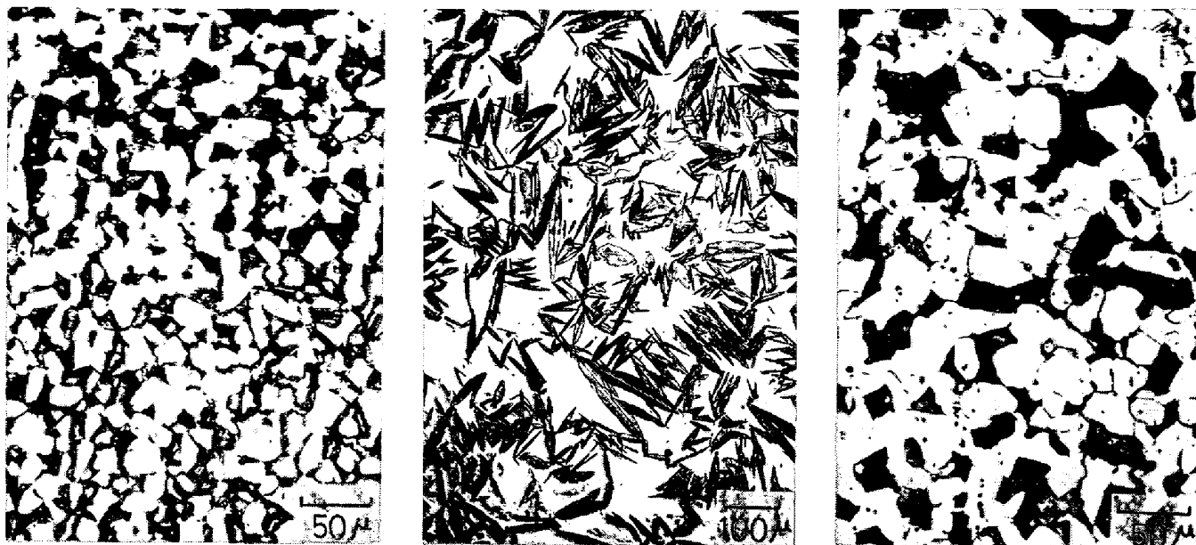
Photo. 1. Optical micrographs of two-phase alloys: (a) Alloy 3 in series A as quenched (A 3 q) containing 51% of ferrite in volume fraction, (b) Alloy 2 of series B (B2) containing 32% of martensite in volume fraction, and (c) Alloy 3 of series C tempered at 600°C (C3 t 600) containing 44% of martensite in volume fraction.
