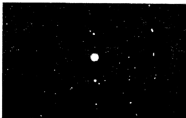
750°C x 10 sec WQ 1 \mu Photo. 5. \gamma formation in \alpha' lath in steel A.
