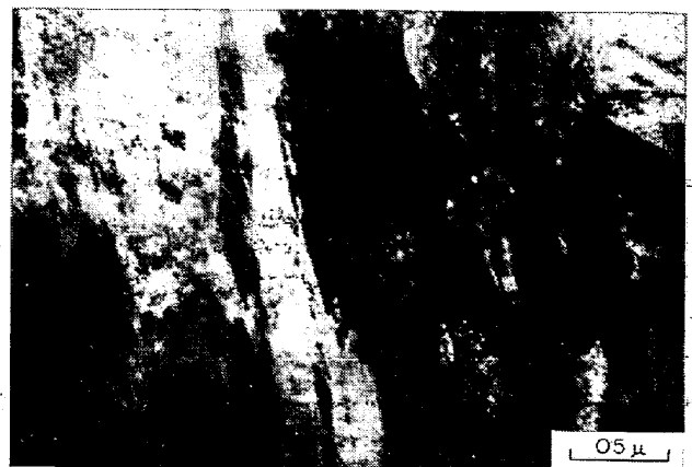
Photo. 10. As quenched structure of non-ausformed alloy M1 (thin foil).
