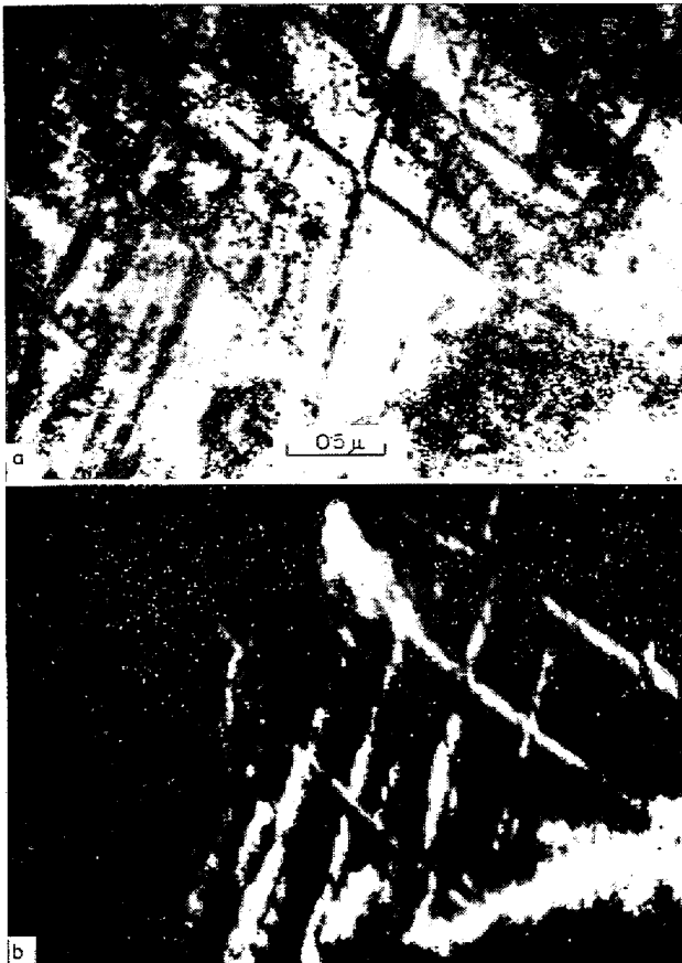
Photo. 3. 5% cold rolled structure of 72% ausformed austenite (alloy S): a) Showing some dark bands formed in austenite. b) Dark field image due to (01\bar{1})_\alpha spot which is arisen from electron diffraction of an area containing dark bands, showing them to be martensite.
