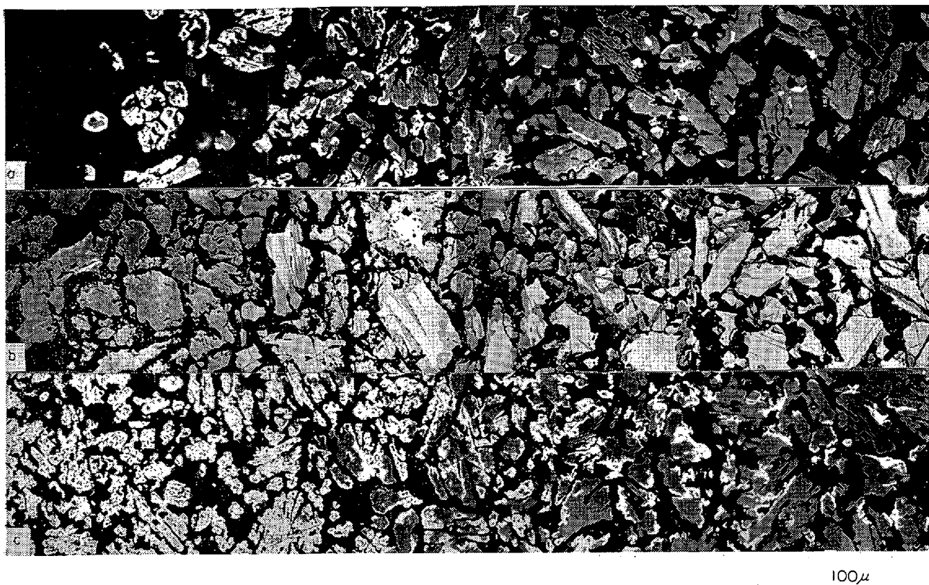
Photo. 2. Microscopic aspects of interfaces of partially reduced pellets at 1100°C. (a) Fe-wustite interface (a part of Photo. 1(b)), (b) Wustite-hematite interface (a part of Photo. 1(b)), (c) Fe-wustite interface (a part of Photo. 1(c)).
