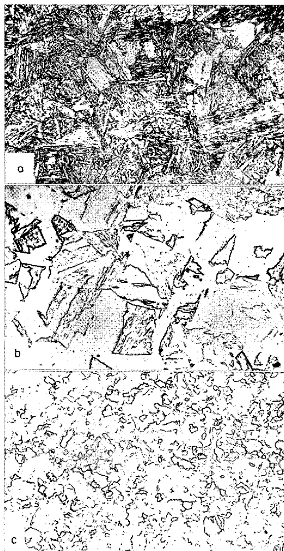
Photo. 1. Microstructures of Fe-5%Ni-0.5%Be alloy water quenched from 950°C. (a) Alloy No 1, (b) Alloy No 2, (c) Alloy No 3. ×240 (2/3)
