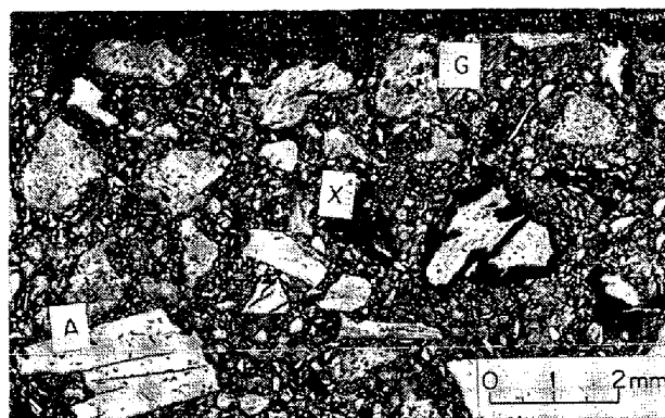
Photo. 3. Microstructure of carbon block oxidized by water vapor at 1000°C —reflected light.
