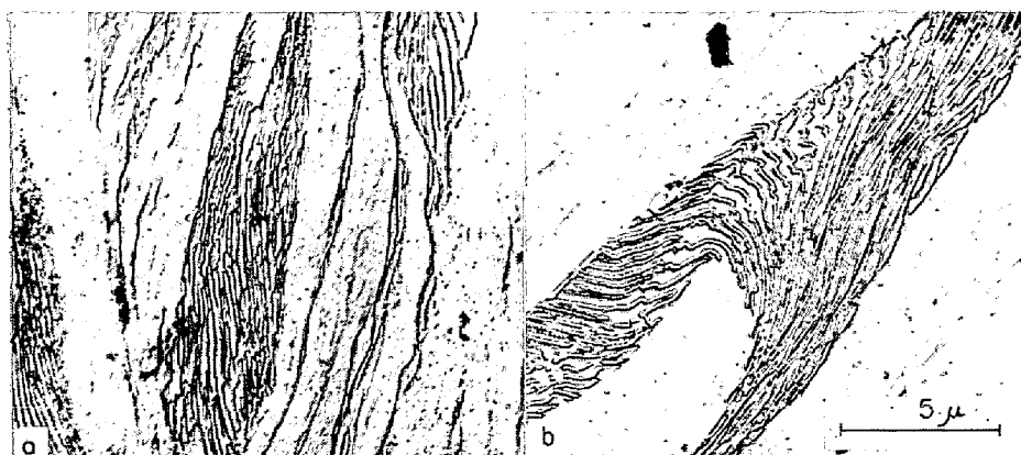
Photo. 3. a) Electron micrograph of deformed pearlite in built up edge (Replica).
