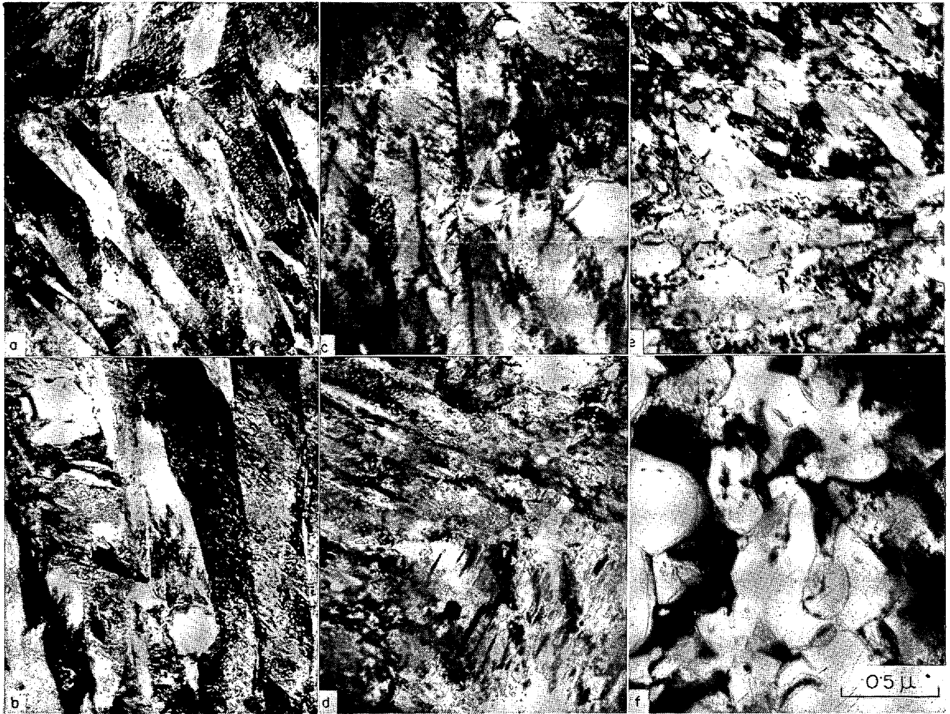
a) Quenched from 830°C b) Quenched from 830°C and tempered at 150°C c) " " 300°C d) " " 400°C e) " " 500°C f) " " 600°C
