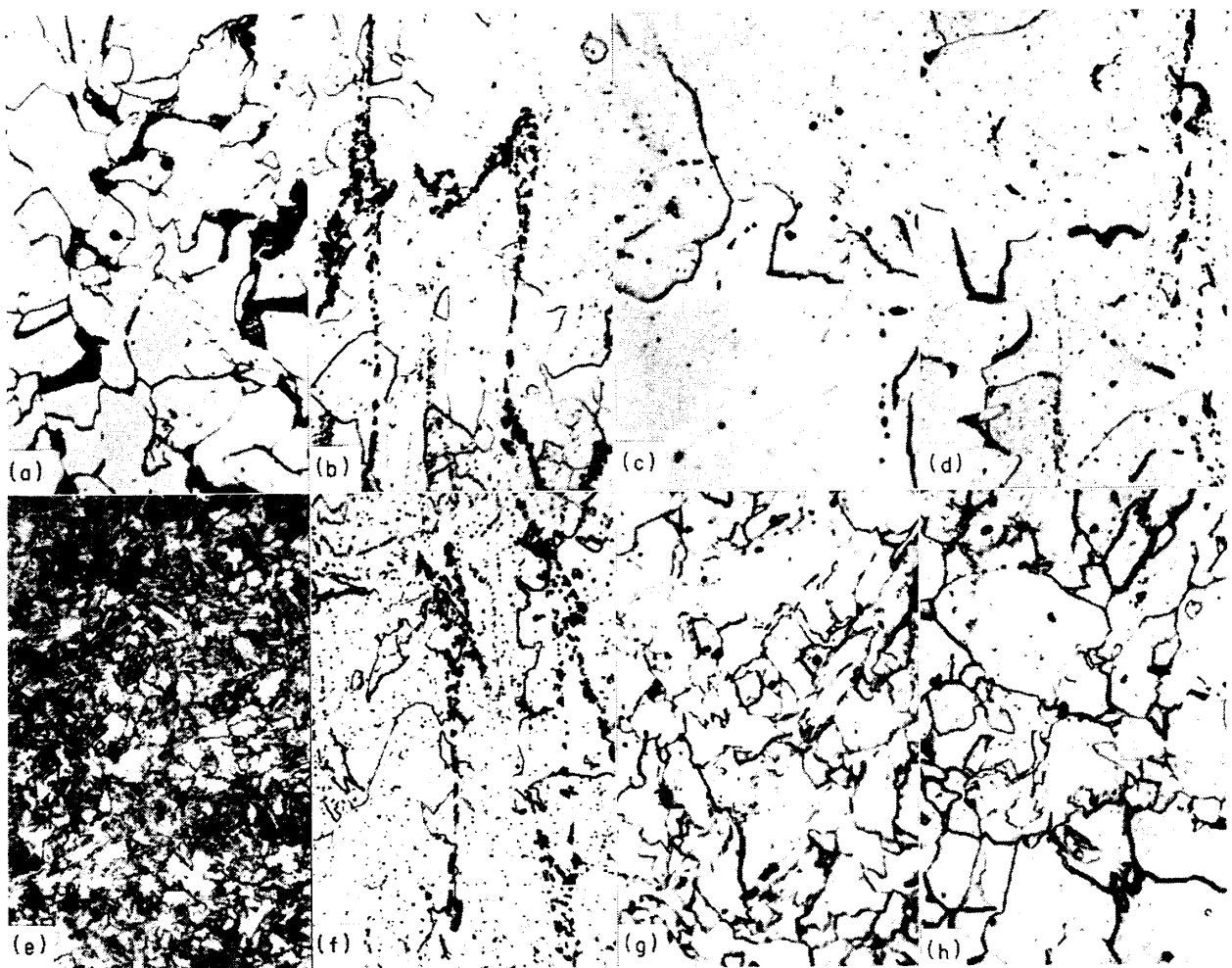
(a) 420A, as forged (b) 420B, as forged (c) 422A, as forged (d) 423A as forged (e) 420A, 1000°C×10hr WQ (f) 420B, 1000°C×10hr WQ (g) 422A, 1000°C×10hr WQ (h) 423B, 1000°C×10hr WQ (×500) 5% picral etched
