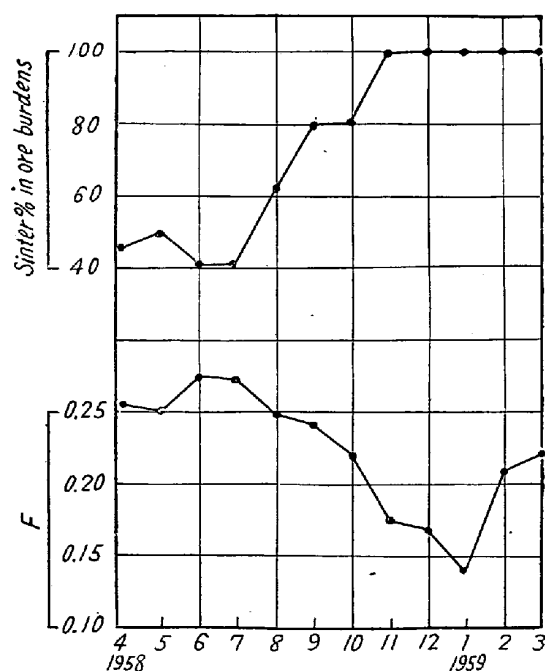
Fig. 2. The changing of resistance of permeability at Kukioka No.2 blast furnace.
