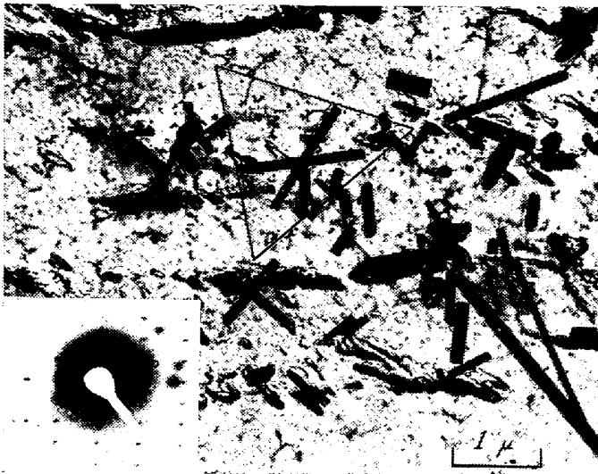
Fig. 3. Extracted AlN by a carbon replica from slow cooled carbon steel (cooled from 1300^{\circ}\text{C} to 900^{\circ}\text{C} at 100^{\circ}\text{C/h} and then water quenched from 900^{\circ}\text{C} , chemical composition is the same as shown in Fig. 1) and electron-diffraction pattern of AlN, AlN particles are larger than in the steel shown in Fig. 1.
