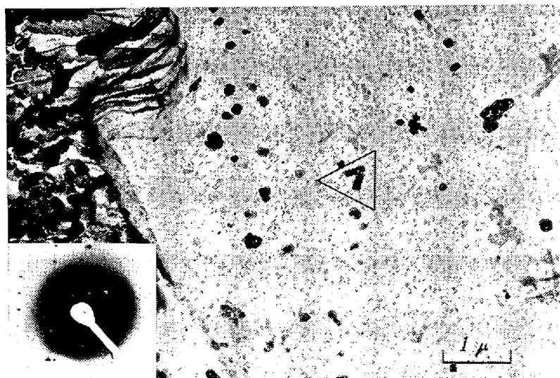
Fig. 2. Extracted aluminum nitride (AlN) by a carbon replica from normalized carbon steel ( 900^{\circ}\text{C} \times 1\text{h} , A. C., C 0.20%, Si 0.24%, Mn 1.37%, soluble Al 0.120%, total N 0.006% and N as AlN 0.003%) and electron diffraction pattern of AlN, AlN particles are smaller than in the steel shown in Fig. 1.
