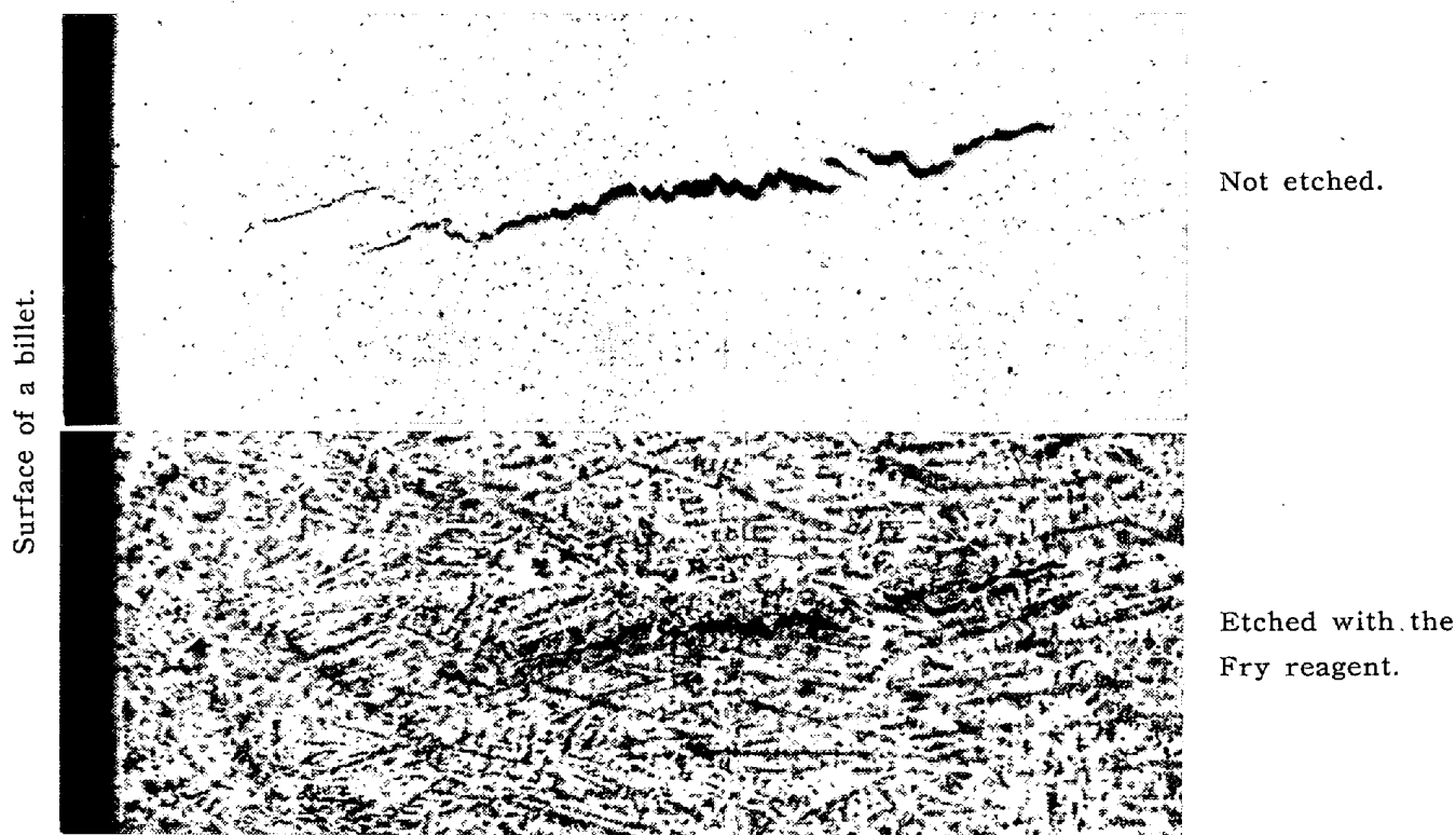
Photo. 4. Transverse section of the longitudinal crack of a billet. \times 30 (2/3)
