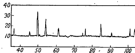
Fig. 1. X-ray diffraction lines of Fe_2O_3 powder Cr(V) , 35KV-6mA, RT \times 1 .
