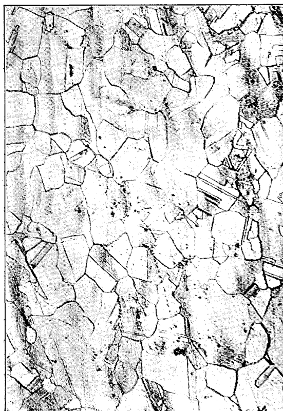
6. Cu 79.5% Ni 19.5 Fe 1.0 (Cu 81.14 Ni 18.68 Fe 0.17(?) Si 0.01 )
